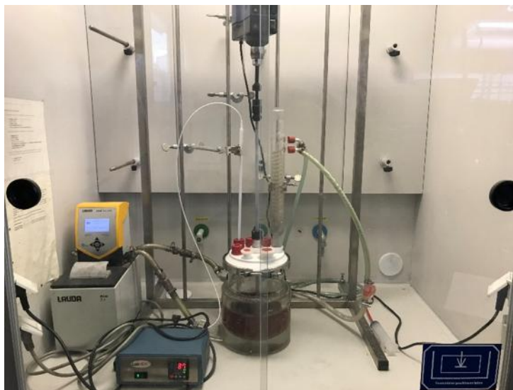
Figure 4. Experimental setup for the leaching experiments.
