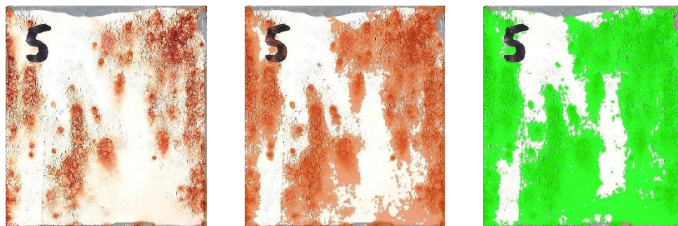
Figure 4. Results of MIPAR analysis with reference images: original corroded surface (left), recipes tailored for each image (middle), overarching recipe (right).
