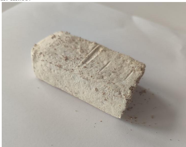
Figure 1. Discarded hazelnut-based biomass used as a precursor for activated carbon.
